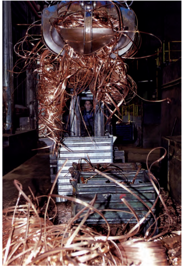
Not just beautiful scrap but first of all valuable recycling material in a variety of shapes: electrical and electronic waste, wires, cable granules and industrial residues containing copper. At the Hamburg plant the copper scrap is pressed into packets weighing up to 600 kg, which are then melted down in the converter.
