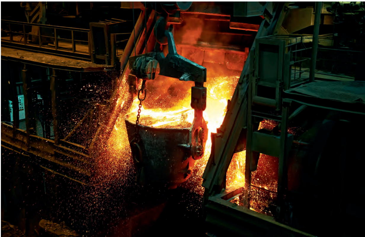
Charging of the converter with copper matte.
