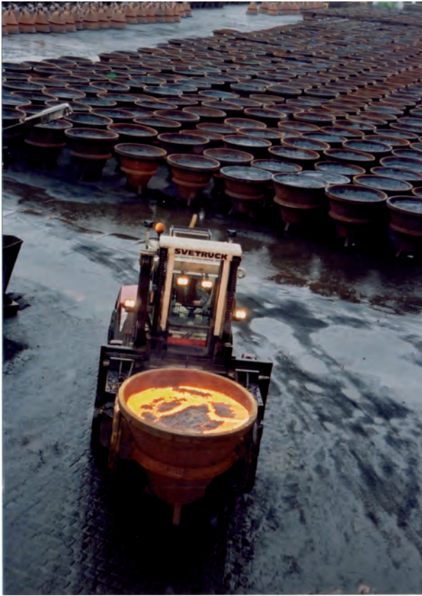
Molds, so-called slag pots, filled with iron silicate stone.
