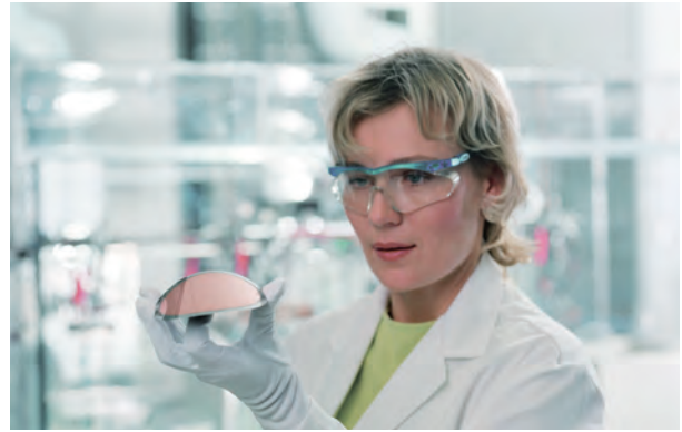
Various patents on solar cell technology were applied for between 1999 and 2002. With the CIS solar technology – copper (C) in combination with the elements indium (I) and selenium (S) – copper offers an efficient alternative to the established silicon solar cells.
