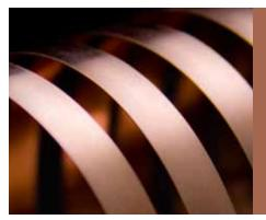
Due to its superior conductivity, Cu-ETP is ideally suited for flat copper conductors, e.g. for the automotive, electrical and photovoltaic industry. Applications include counter helix strip, finned tubes and connectors. Aurubis offers material with different tensile strengths, thicknesses and widths depending on the width/thickness ratio.
